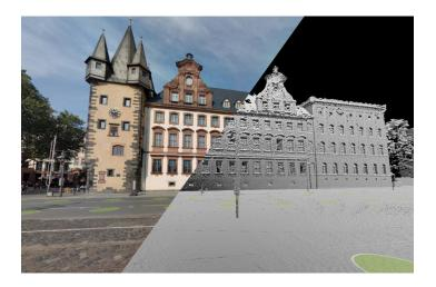
The depth information available in the 3D-Cyclorama allows you to measure with the Measure Smart function without having to make a forward cut. This means that a 3D measurement can be carried out with just one click.
