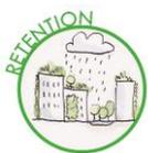
Rainwater is retained to reduce the risk of flooding, reduce surface water flows, reduce stress on stormwater sewers, and restore natural hydrology. | <ul style="list-style-type: none"> <li>• Rooftop retention by blue /green roofs</li> <li>• (Collective) raingardens</li> </ul>                                                                                                                                                                                                                              |
