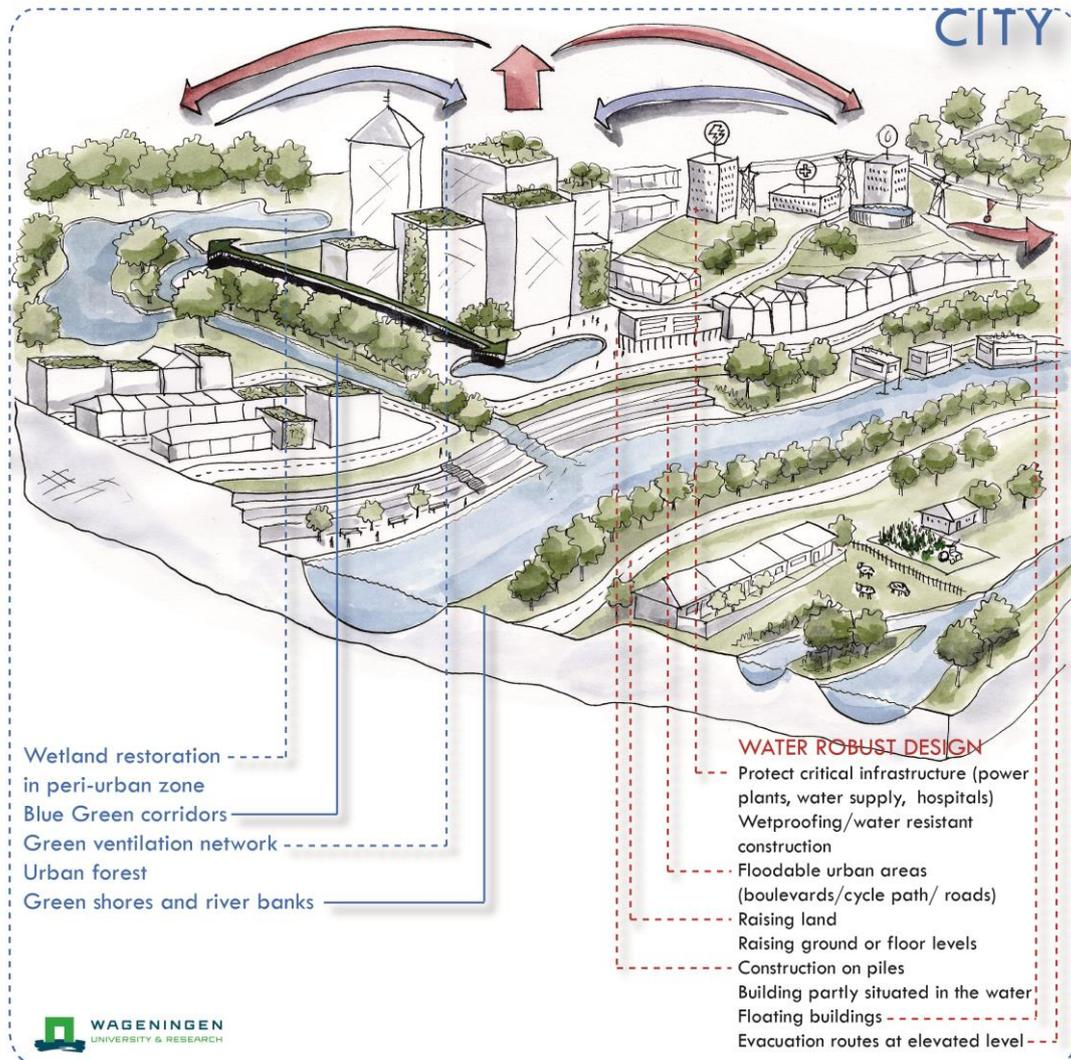
Figure 3.4 Illustration of possible Water Smart measures on city scale
