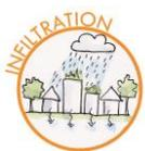
Infiltrate rainwater into the ground                                                                                                                 | <ul style="list-style-type: none"> <li>• Reduced paved surface</li> <li>• Create more green space</li> <li>• Infiltration zones/trenches</li> <li>• Infiltration sewer / well</li> <li>• Disconnect paved surface from sewer system</li> <li>• Permeable paving</li> <li>• Wadi / bioswales/Tree pit</li> <li>• Geocellular/infiltration systems</li> </ul> |
