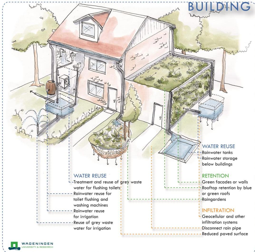
**Figure 3.2 Illustration of possible Water Smart measures on building scale**
